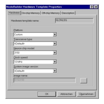
In the above screenshots you can see all the necessary NodeBuilder Hardware Template settings that have to be done for the **EXLON**\*\*.
